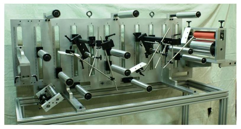
Create a custom converting line with your existing equipment by adding a Telstar Plow Fold Unit for booklet and coupon production. Units are available for Single, Double, and Triple folds. Telstar Plow Fold units can be engineered to bolt inline to virtually any press.
